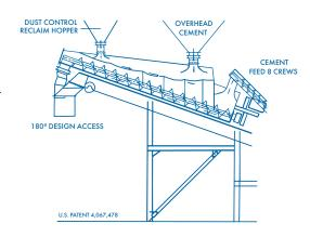
The live-bottom aggregate batcher delivers precise proportions of sand and aggregate during discharge. The variable speed drive maintains a constant rate of discharge throughout the discharge cycle. And the unique inverted V-trough above the conveyor belt reduces belt wear and excessive starting load.
